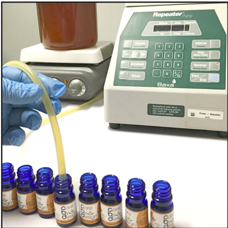
PERISTALTIC PUMP releases uniform amounts of cannabinoid-rich mixture through tube to fill sublingual spray bottles. Beaker at left contains essential oil with one of five CBD-to-THC ratios, mixed with coconut oil. Magnetic stir plate keeps the blend well-mixed throughout the process.
