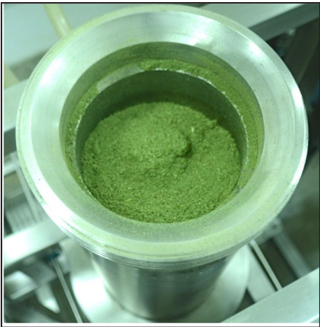
EXTRACTION VESSEL is packed full of dried cannabis that has been very finely grated through a stainless steel screen. The vessel, manufactured by machinists employed by Critical Solutions, is six inches in diameter and four feet deep. It holds 20 liters — typically, six pounds of ground cannabis, which will yield about three liters of essential oil.
