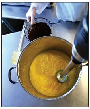
EMULSIFICATION is the physical mixing of liquids that are normally immiscible. The stainless steel bowl holds eight gallons, the mixer is a 750-watt commercial Immersion blender. Hand-crafted batches are made two to four gallons at a time.
