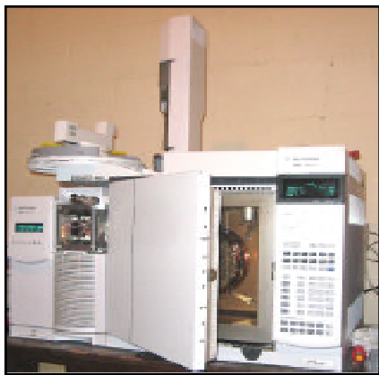
GAS CHROMATOGRAPH/MASS SPECTROMETER consists of two instruments that work together in tandem. The GC (unit at right with open door) is used to measure quantities of known compounds. As sample is heated very slowly in “oven,” molecules rise into vertical column and cling to walls at identifiable levels. MS unit at left identifies unknown substances.
