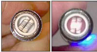
VAPE PEN HEATING ELEMENT (left) turns red-hot in seconds. "This is burning, not vaporizing," said Russo. Vape pens using propylene glycol as a propellant have been shown to produce cancer-causing formaldehyde. PHOTOS BY ETHAN RUSSO
