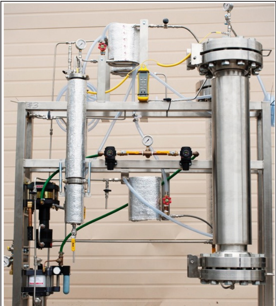
SUPERCRITICAL FLUID EXTRACTION UNIT has a 4-foot tall flanged extraction vessel (right) that that can hold 20 liters. Smaller separator vessels are on left.
