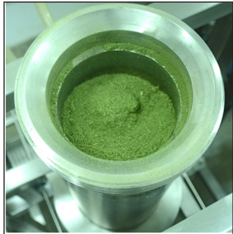
EXTRACTION VESSEL is packed full of dried cannabis that has been very finely grated through a stainless steel screen. The vessel, manufactured by machinists employed by Critical Solutions, is six inches in diameter and four feet deep. It holds 20 liters — typically, six pounds of ground cannabis, which will yield 200-300 grams of essential oil.
